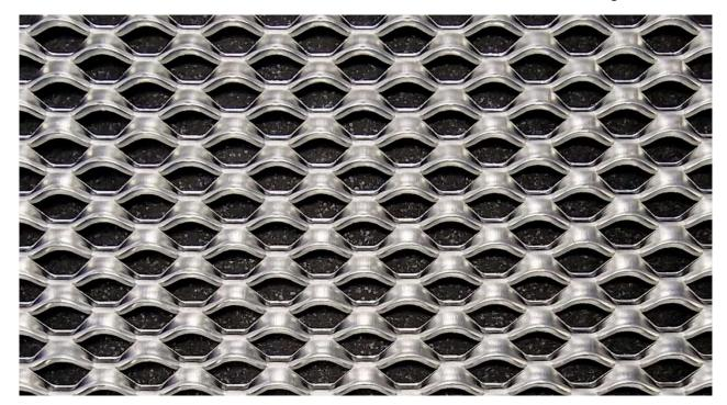
LW Pitch:20.00mmStrand Width:4.00mmSW Pitch:13.00mmThickness:2.00mmWeight:3.32 kg / m2Open Area:38%
